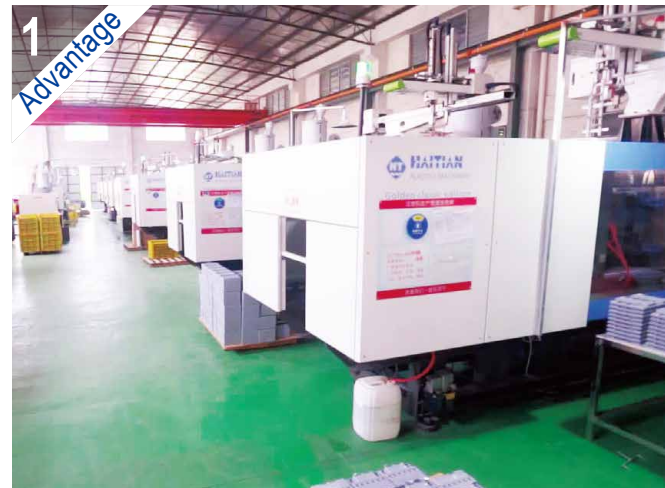
➤ Battery Case injection process Fresh ABS raw material. Cases are injected by JYC, insuring battery cases quality from the source.
