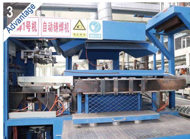
➤ Cast-Welding Automatic plates-group cast-welding technique insures stable welding to the battery, without disconnection.
