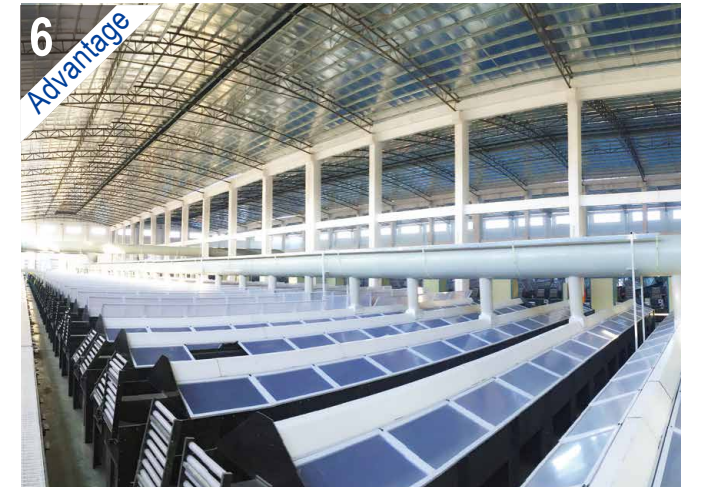
➤ Inner formation Advanced and proven inner formation technique prevents the batteries from electrolyte emission, insuring plate formation complete and enabling batteries longer lifetime.
