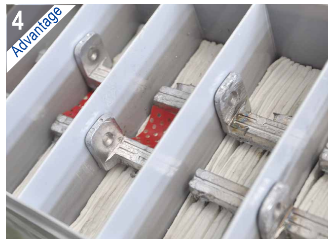
➤ TTP-Welding(Through The Partition) Automatic TTP machines and proven technique insure battery quality, reducing battery internal resistance, decreasing labor and material costs.
