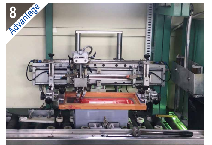
➤ Automatic packing line Automatic silkscreen-printing and packing lines insure stable printing quality and decrease labor costs.
