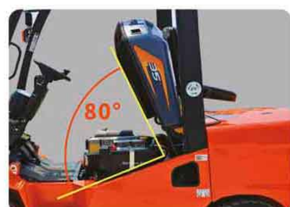
The engine hood opens at an 80-degree angle.
