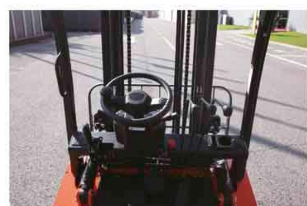
The widened mast provides a better field of vision.
