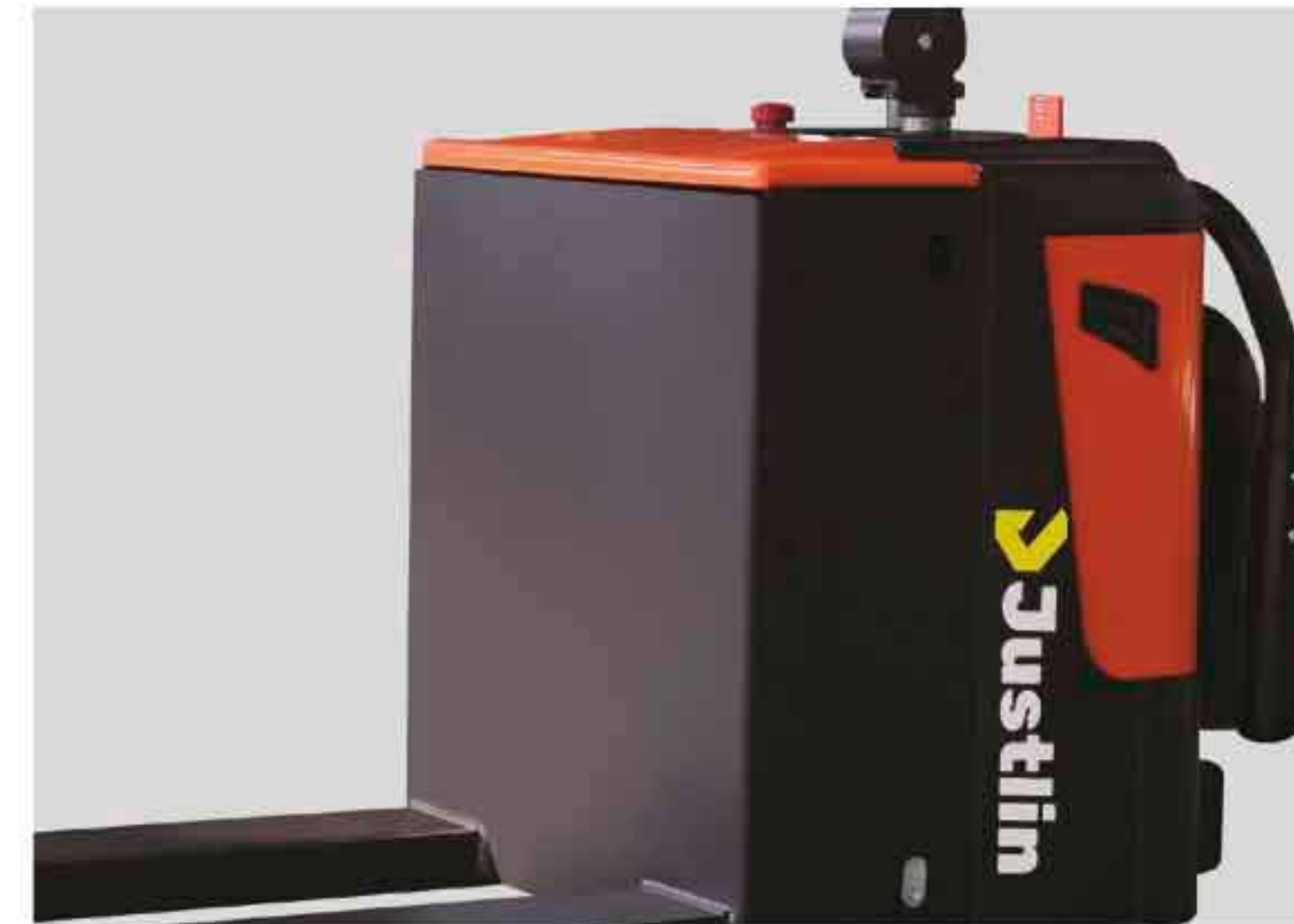
Robust design Reinforced metal battery cover and body casing.
