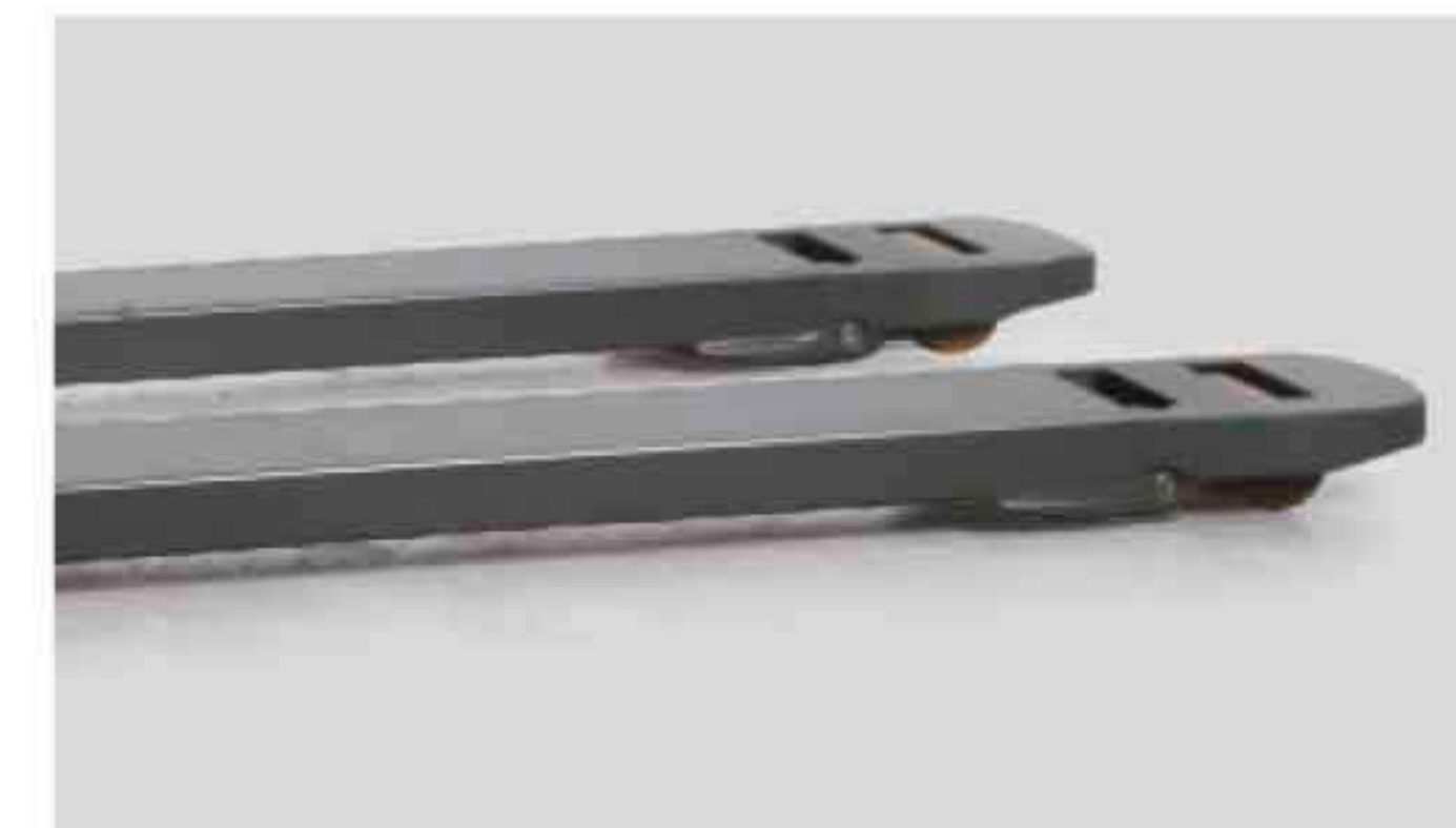
Optional American-style components American-style fork carriage with short fork tips.
