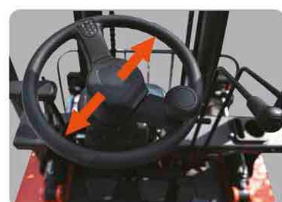
A smaller diameter steering wheel is used to reduce operator fatigue.
