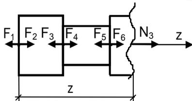
$$\begin{aligned} \Sigma z=0 \quad N_3 - F_1 + F_2 - F_3 + F_4 - F_5 + F_6 &= 0 \\ N_3 = F_1 - F_2 + F_3 - F_4 + F_5 - F_6 &= \\ = 24 - 20 + 36 - 10 + 0 - 12 &= 18 \text{ кН} \\ \sigma_3 = N_3 / A_3 &= 18 / 2.26 = 7.962 \text{ кН/см}^2 \end{aligned}$$
