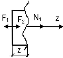
$$\begin{aligned} \Sigma z=0 \quad N_1 - F_1 + F_2 &= 0 \\ N_1 = F_1 - F_2 &= 24 - 20 = 4 \text{ кН} \\ \sigma_1 = N_1 / A_1 &= 4 / 15.83 = 0.253 \text{ кН/см}^2 \end{aligned}$$
