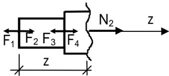
$$\begin{aligned} \Sigma z=0 \quad N_2 - F_1 + F_2 - F_3 + F_4 &= 0 \\ N_2 = F_1 - F_2 + F_3 - F_4 &= 24 - 20 + 36 - 10 = 30 \text{ кН} \\ \sigma_2 = N_2 / A_2 &= 30 / 6.03 = 4.976 \text{ кН/см}^2 \end{aligned}$$
