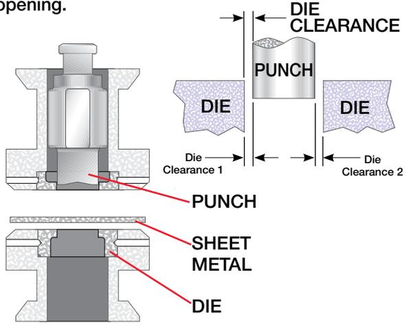
Total Die Clearance = Die Clearance both sides of Punch
