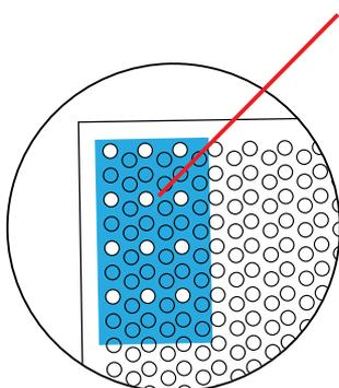
**PUNCHING FORCE FORMULA** = linear length of cut x material thickness x shear strength = punching force in kilonewtons(kN).
