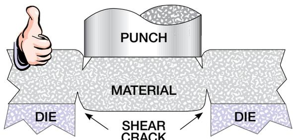
**OPTIMUM CLEARANCE** – shear cracks join, balancing punching force, piece part quality and tool life.
