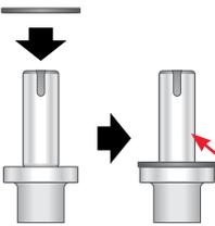
Place spring washer over punch shank onto punch shoulder. Apply lubricant to punch shank.
