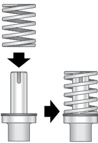
Place spring over punch shank on top of washer.
