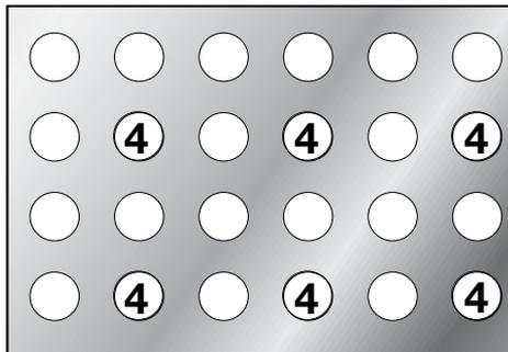
For greater hole uniformity and flatter sheets, spread the punches to avoid punching adjacent holes in the same hit. Complete the desired pattern with the technique known as bridge hitting.
