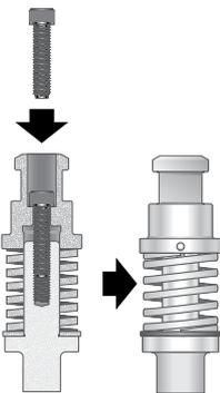
Insert 6mm socket head cap screw through tang and lightly tighten to the punch with a 5mm hex wrench - approximately 8 revolutions. Note: cap screw must not be over tightened at this step. Over tightening may result in misalignment during assembly.
