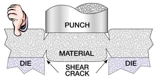
**CLEARANCE TOO SMALL** – secondary shear cracks are created, raising punching force and shortening tool life.
