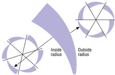
This tool's large radii results in blanks with smoother edges produced with fewer hits than with an ordinary radius punch. This tool can be programmed to punch holes with slugs or parts retained in the sheet, yet can be separated easily off the press.
