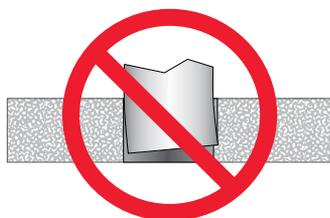
**DO NOT DOUBLE-HIT HOLES.** Using the cluster punch to finish missed holes in patterns will cause punches to shave sides of previously punched holes. The great lateral thrust from this shaving shortens punch life. Use a single-hole punch to complete the pattern.
