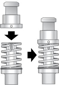
Place tang onto punch shank so that internal locating pin is visually in line with punch angle orientation slot.
