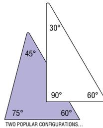
The 3-way notching tool can include angles from 150° to 15° - shown above are two popular arrangements. One tool can provide nine corner options - with auto index in two hits.
