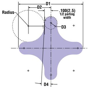
The 4-way corner rounding tool can round all four corners of a piece part without rotating the tooling - use with standard parting tools for piece part separation.
