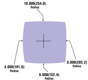
The quad radius tool nibbles large holes with smoother edges and fewer hits than using a round nibbling punch. In effect, smooth round holes not limited to station range.
