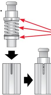
Apply lubricant to outside surfaces of punch shoulder, spring, and tang flange.
