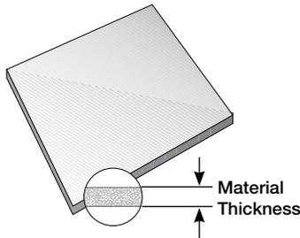
Material thickness is the width of the workpiece or sheet that the punch must penetrate in making a hole. Generally the thicker the material the more difficult it is to punch, but this isn't the only factor.
