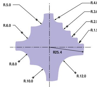
A single 9-way corner rounding tool provides nine popular radii in one tool. Auto indexing selects and rotates the desired radius to round off all corners of a piece part.
