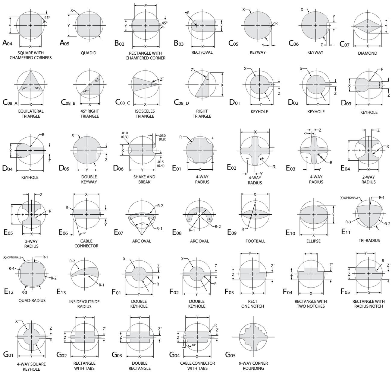
When ordering a special shape, please provide all dimensions noted above for the corresponding shape. Special shape drawings are also available on [mate.com](http://mate.com).
