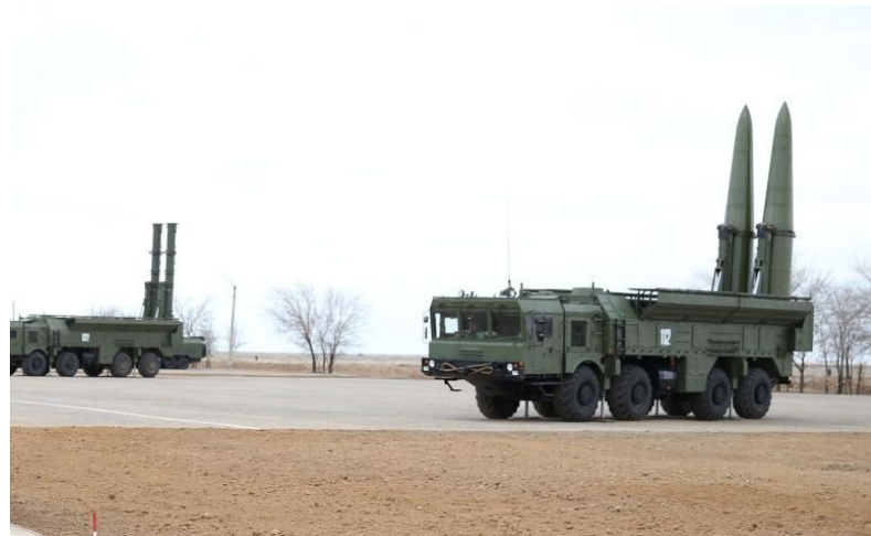
The 9K720 Iskander (NATO: SS-26 Stone) — a road-mobile short-range ballistic missile (SRBM) with a range of up to 500 km
